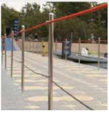
Fixed 50 cm back from the edge like traditional center pin Mounted on 1 center pin - Weight : 4,00 kg Dimensions : Ø x H : 4,2 x 110 cm - Marine quality stainless steel Distance between each rail from 2 m to 3 m – linked by 16 mm red/orange ropes as handrail (sold separately)
