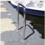
Fixed 50 cm back from the edge like traditional center pin Mounted on 2 center pins - Weight : 8,00 kg Dimensions : Ø x H : 4,2 x 110 cm - Marine quality stainless steel Mainly used for boarding passengers
