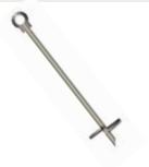
1 plate galvanized – dimensions 1.25m x30mm 1 plate 250x10 Installation in loose soil (sand, mud, loose soil)) Tensile strenght 1 T (depending of the ground) mechanical or manual installation
