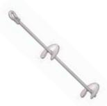
2 plates galvanized – dimensions 1.5m x30mm 2 plates 250x10 Installation in loose soil (sand, mud, loose soil)) Tensile strenght 2 T (depending of the ground) mechanical or manual installation
