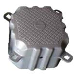
Size: L x I x H: 50 x 50 x 40 cm - Weight: 6,50 Kg - Buoyancy: 91,5 Kg Resistance of assembling rings: 2.000 Kg - Patented male/female interlocking system Shockproof PEHD (High Density Polyethylene) - Antistatic, low flammability Standard colours: beige and light grey - Other colours on demand (1 000 pieces minimum). Anti-skid structure - Based on 4 plots (increase stability, reduce current pressure) - ECO Patented
